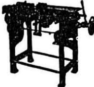
This PETERS JUNIOR CARTON FOLDING AND CLOSING MACHINE closes 35-40 "Peters Style" cartons per minute. Requires no operator.
